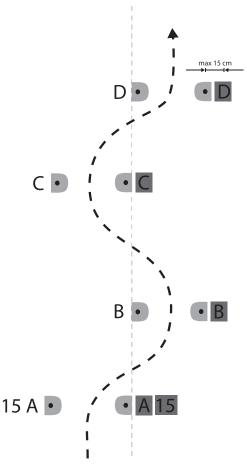
Centerline cones to be set in a straight line, either in front, at the middle or at the rear of the cone (as shown above) with markers placed within 15cm.
