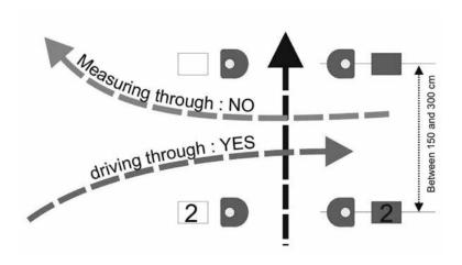
Distance between the two pair of cones: minimum 1.5, maximum 3 metres.
